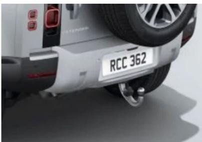
Electrically Deployable Tow Bar
